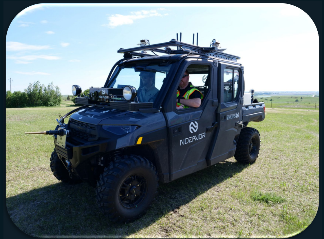
NDeavor semi-autonomous UTV in field testing
