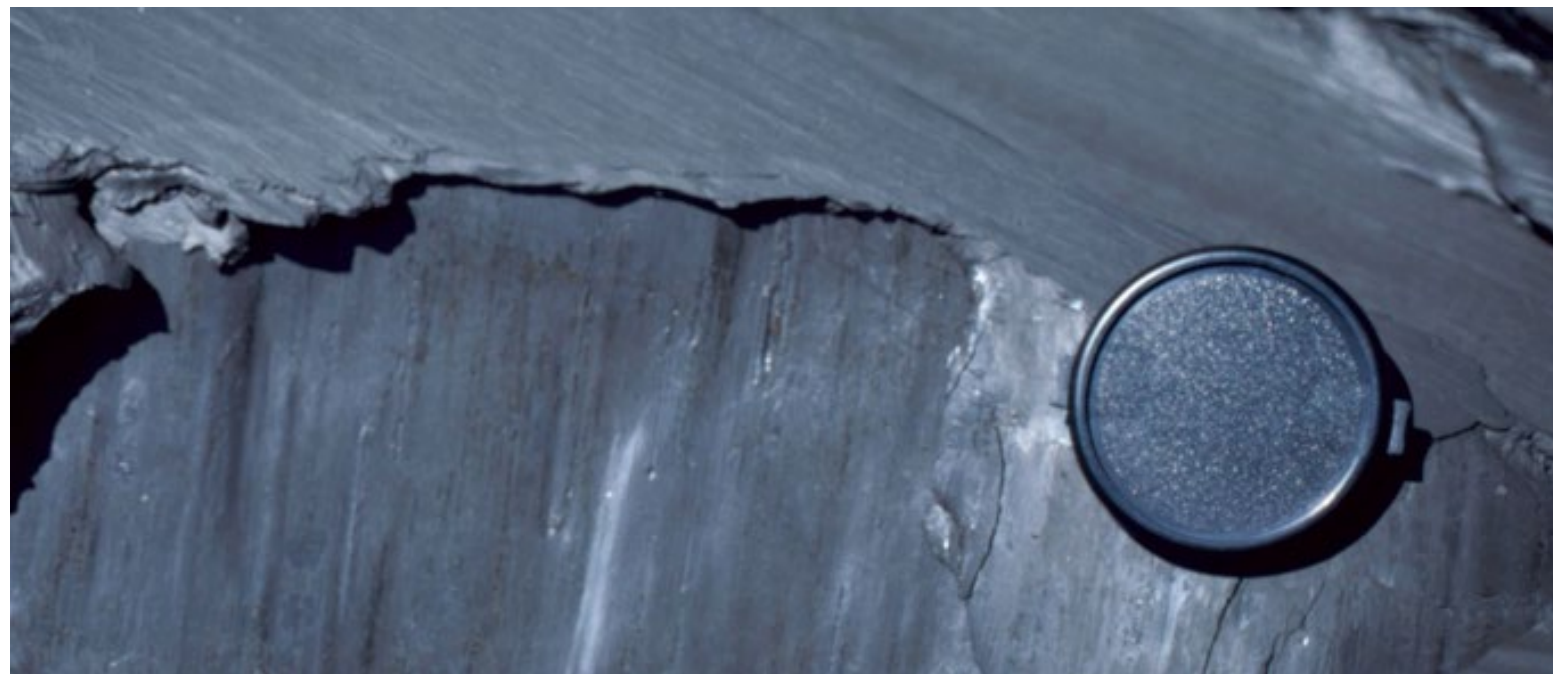
Photograph of the soft and expansive lake clay of the Brenna Formation found in the shallow subsurface of the Fargo area. The lineations on the face of the sample are called “slickensides” or “slicks” which shows how this clay can deform under pressure. This sample was photographed during construction of the Fargo landfill.
