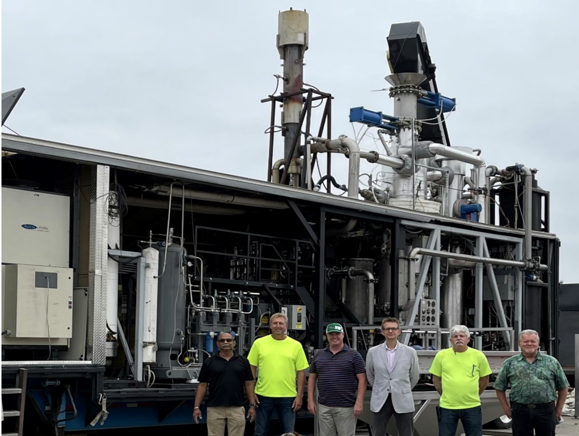
Figure 3. Teams from Dakota Green Power and the City of Grand Forks shown together with Tri-Steel's 5 ton/day truck-mounted Sandwich Gasifier.
