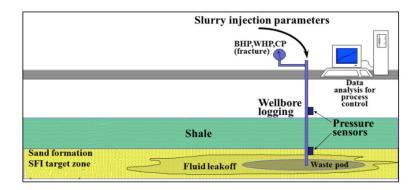
The fluid rapidly dissipates into surrounding the formation allowing injection pressure to disappear quickly. This leaves no long-term remnant of pressurization. The solid waste remains behind, entombed permanently by the weight of the
