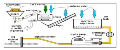
On the surface, the waste streams are mixed into a slurry with an aqueous carrier fluid using a surface processing unit. This slurry is introduced into a reciprocating slurry pump capable of achieving high pressures and pumped into the wellbore.
