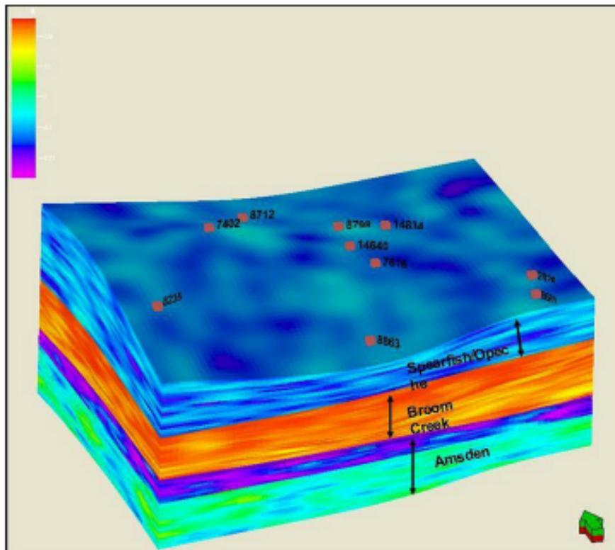
Figure 7. CO<sub>2</sub> storage potential in the Broom Creek aquifer in the bigger Washburn area.
