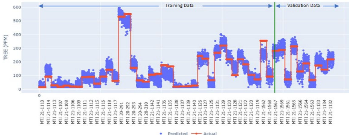
Figure 2. Ore analysis algorithm training/validation from MTI's previous development using PGNAA-DGA
