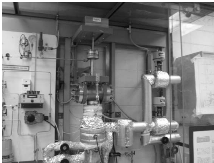
Figure 2.6.4. Photograph of the Subpilot-scale U-GAS® Gasifier to be Used in the Study.
