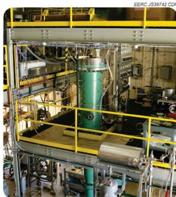
Figure B-7. Schematic and photograph of the bench-scale EFG.
