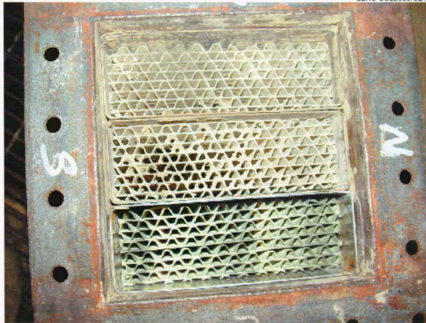
Figure 9. Catalyst ready for the SCR reactor assembly. Two physically cleaned, previously exposed catalysts at the top, new catalyst at the bottom; Coyote Station at the 2-month test interval.
