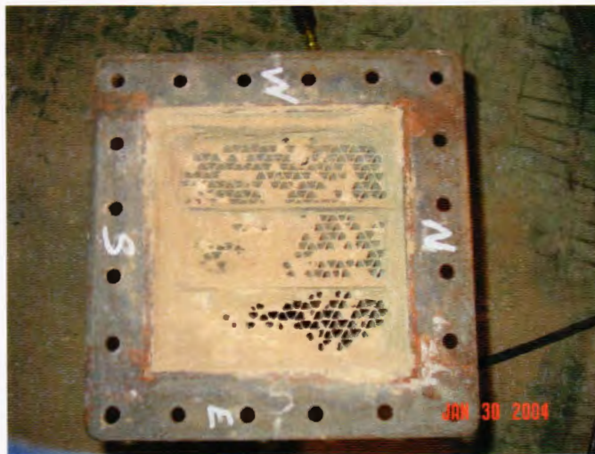
Figure 31. Pictures of catalyst inlet after about 4 months of exposure to flue gas and particulate.
