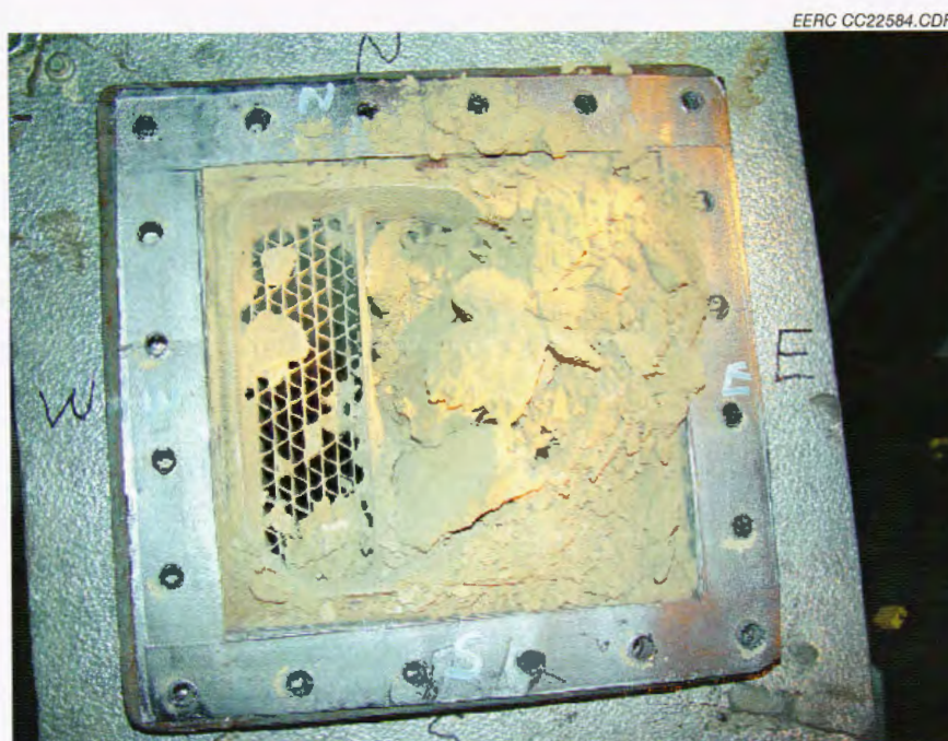
Figure 5. Inlet of the SCR catalyst section after 2 months of field testing at the Coyote Station.
