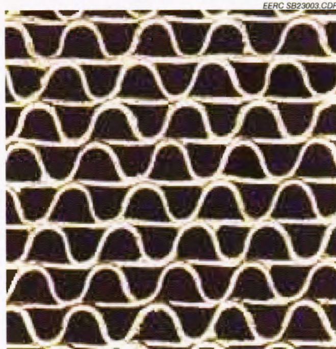
Figure 19. Haldor Topsoe SCR catalyst showing the gas flow passages.
