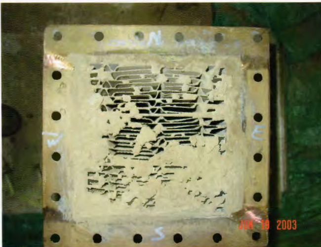
Figure 30. Pictures of catalyst inlet after about 2 months of testing at each plant.
