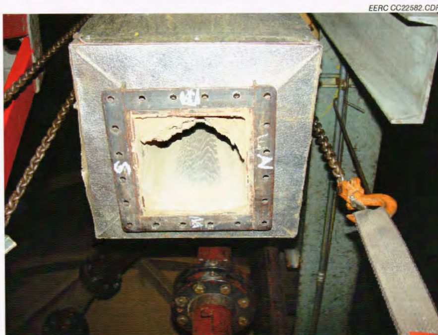
Figure 3. Inlet to the catalyst section of the SCR reactor view looking upstream; Coyote Station at the 2-month test interval.
