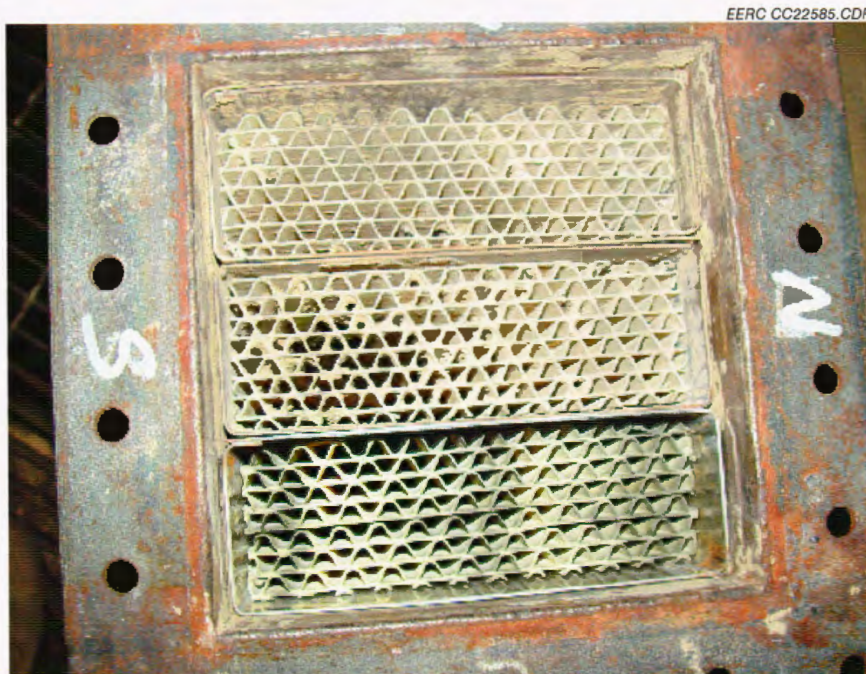
Figure 8. Catalyst ready for the SCR reactor assembly. Two physically cleaned, previously exposed catalysts at the top, new catalyst at the bottom; Coyote Station at the 2-month test interval.
