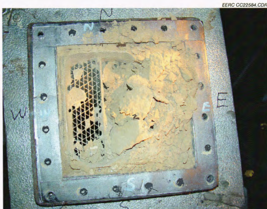
Figure 6. Inlet of the SCR catalyst section after 2 months of field testing at the Coyote Station.
