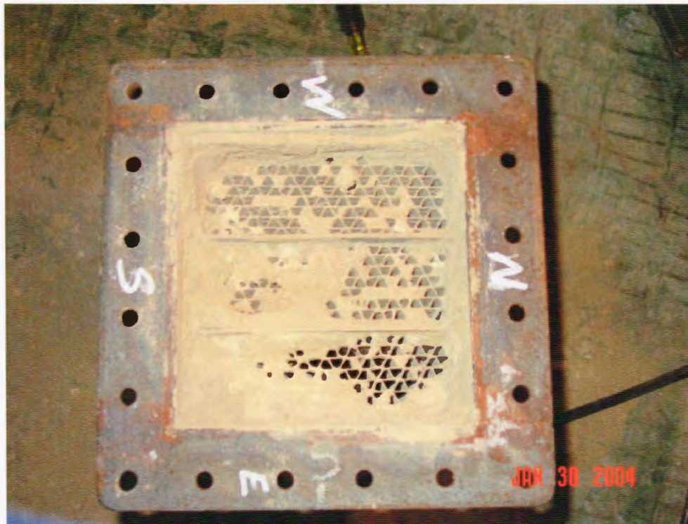
Figure 5. Pictures of catalyst inlet after about 4 months of exposure to flue gas and particulate. The top is the Haldor-Topsoe catalyst from Baldwin Station; the bottom is the Haldor-Topsoe catalyst at Coyote Station.
