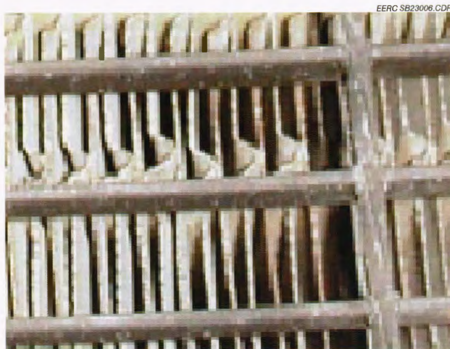
Figure 20. Babcock Hitachi SCR catalyst showing the gas flow passages.
