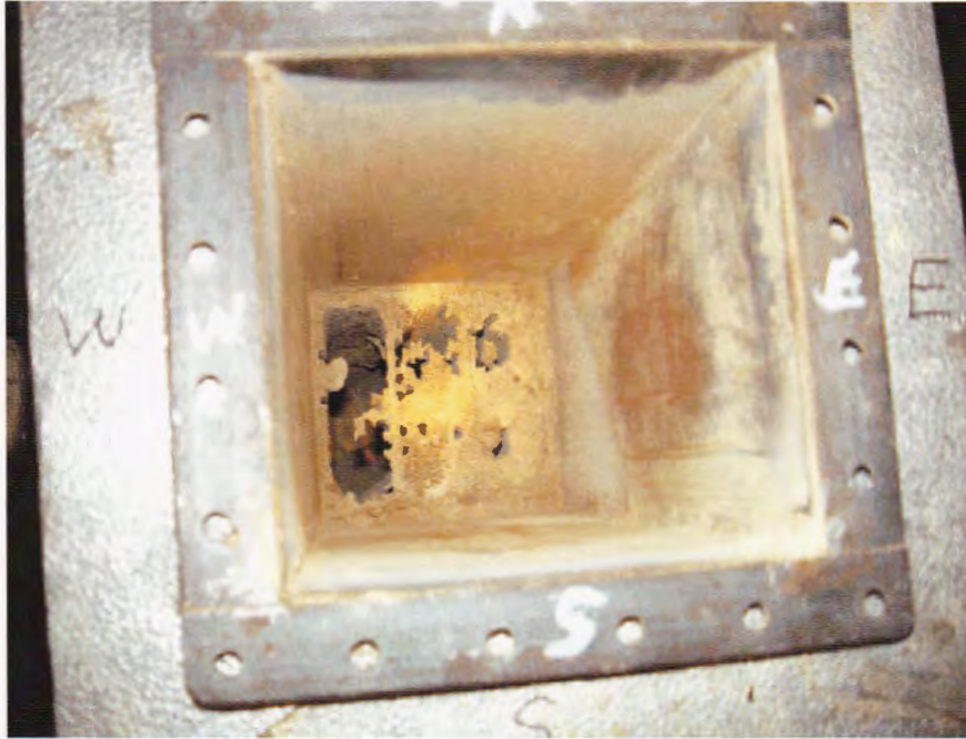
Figure 8. Inlet of the catalyst section of the SCR reactor after catalysts have been removed; view looking downstream; Coyote Station at the 2-month test interval.
