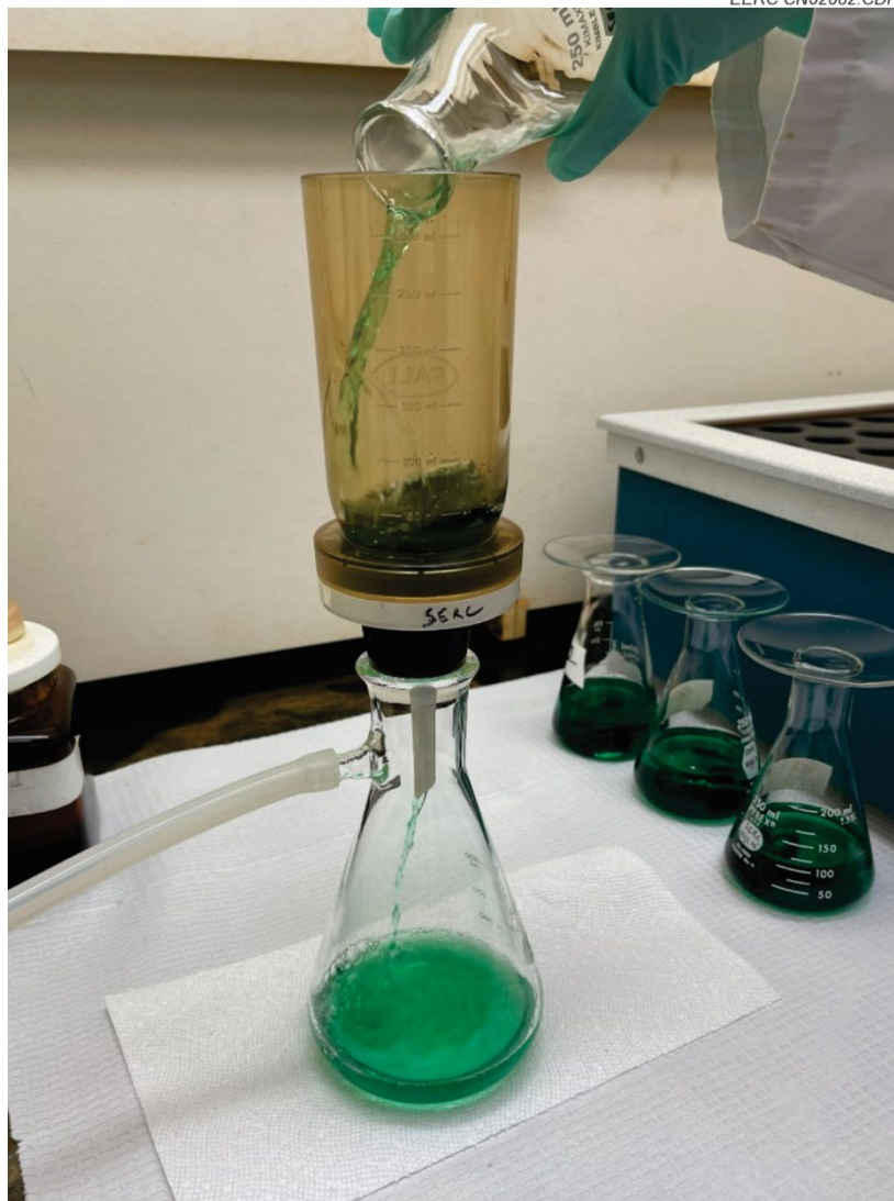
Figure 5. Concentrated PGE precipitate is separated before being prepared for inductively coupled plasma–mass spectrometry (ICP–MS) analysis.
