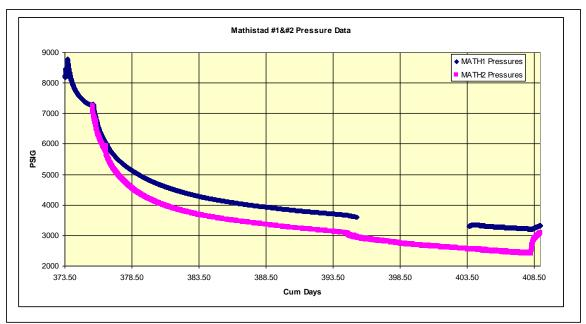
Figure 13 #1 & #2 Pressure data during flowback of the #2
