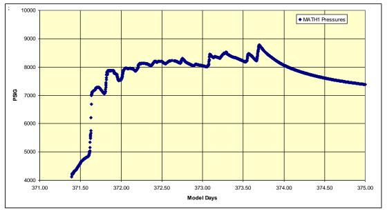
Figure 11 Mathistad #1 BHP during the #2 frac showing bumps in pressure from the 14 frac stages.
