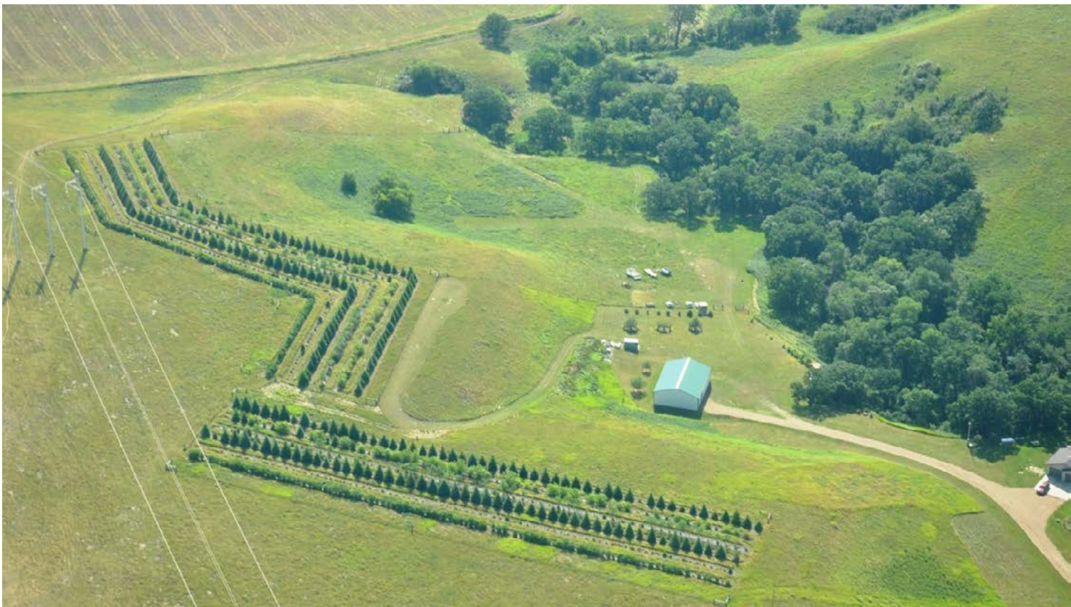
Living snow fences protect rural homes and stretches of highway from blizzards.
