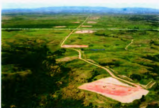
Well sites placed along energy corridors (shown above) help keep development and traffic confined to one area. Horizontal drilling allows companies to drill under sensitive habitat, reducing or eliminating disturbance to critical species. Photo courtesy of Vern Whitten.
