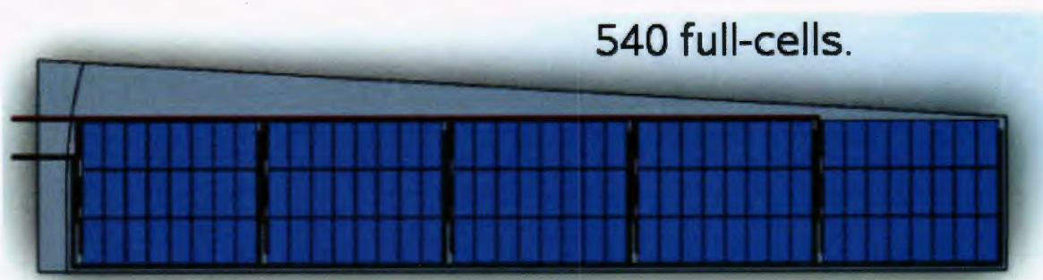
Figure 2: Inner Section of SBXC Wing with Solar Cells
