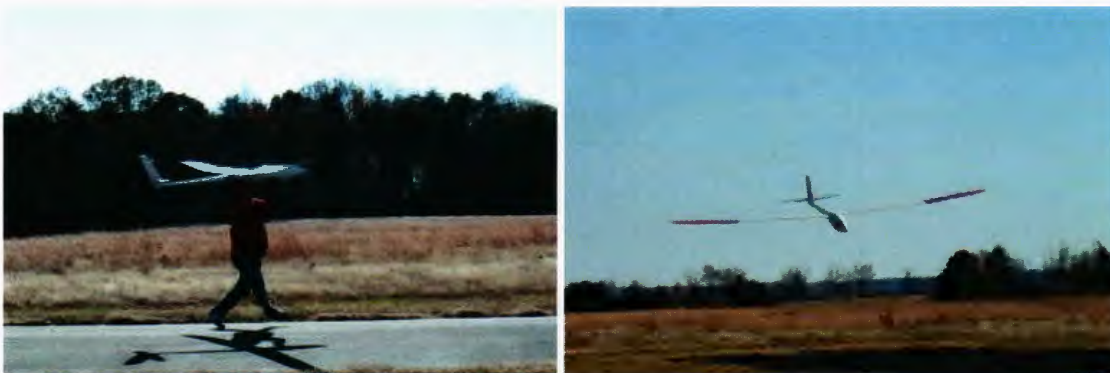
Figure 11: Prototype SBXC hand-launched takeoff (left) and belly-landing (right).
