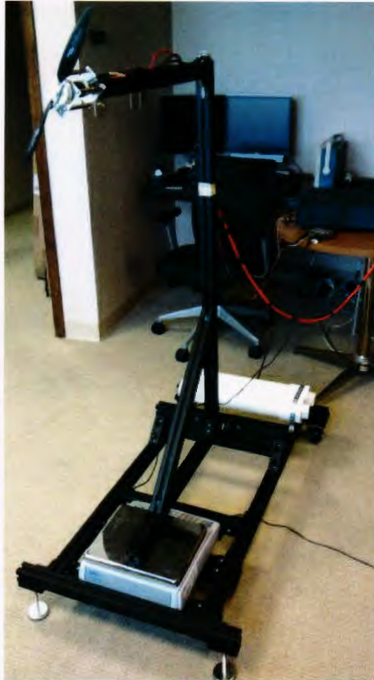
Figure 22: Thrust Measurement Stand
