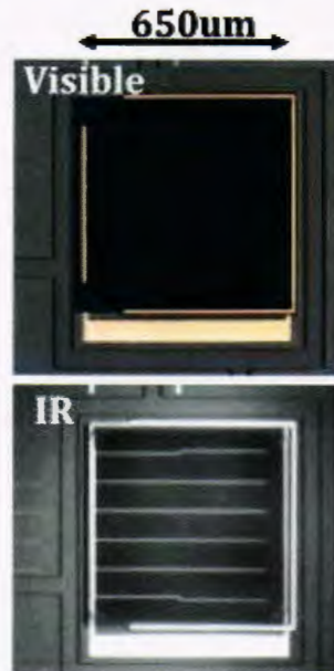
Figure 2: Photograph of a stacked cell. Top picture (visible) shows the GaAs-based cells, the bottom figure (IR) shows the bottom, InP cells.
