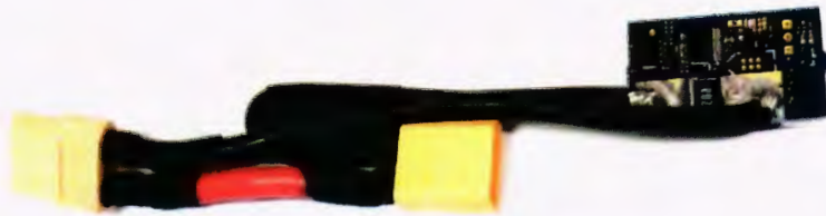
Figure 11: Inline Battery Monitor
