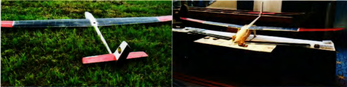
Figure 6: These are photos of the UAS with the Si solar cells integrated onto the wing skin. The solar arrays consists of full sized and custom made cells, built at NRL.
