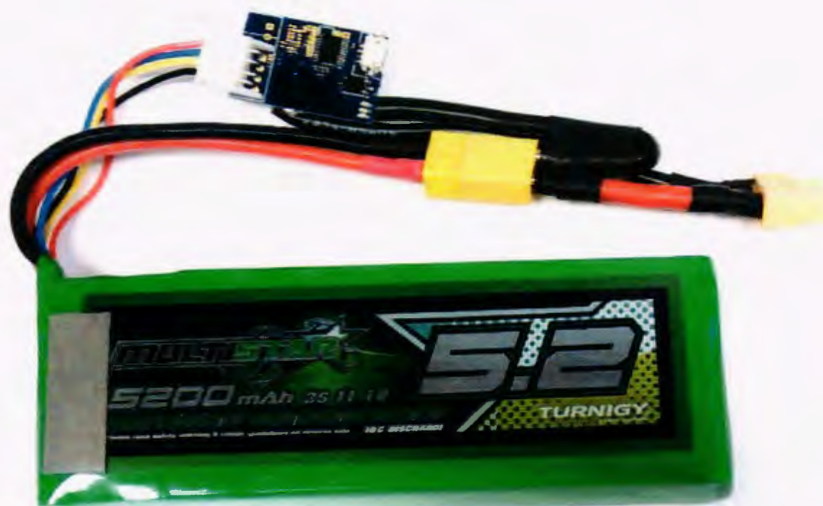
Figure 12: Inline Battery Monitor with Battery Pack
