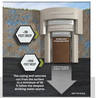
As required under the permit to drill, groundwater resources are protected during drilling by freshwater drilling mud, then isolated with layers of steel casing and concrete The casing and cement remain as permanent protection for groundwater; see "Drill the Hole" on the back page for more details.
