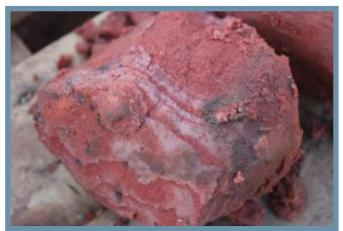
A rock core cut from the target CO2 storage layer 6400 feet below ground shows the pink sandstone of the Broom Creek Formation. It has the consistency of playground sand.
