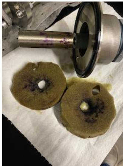
Figure 7: Foam and Electrode condition after 10KV- 50 °C application
