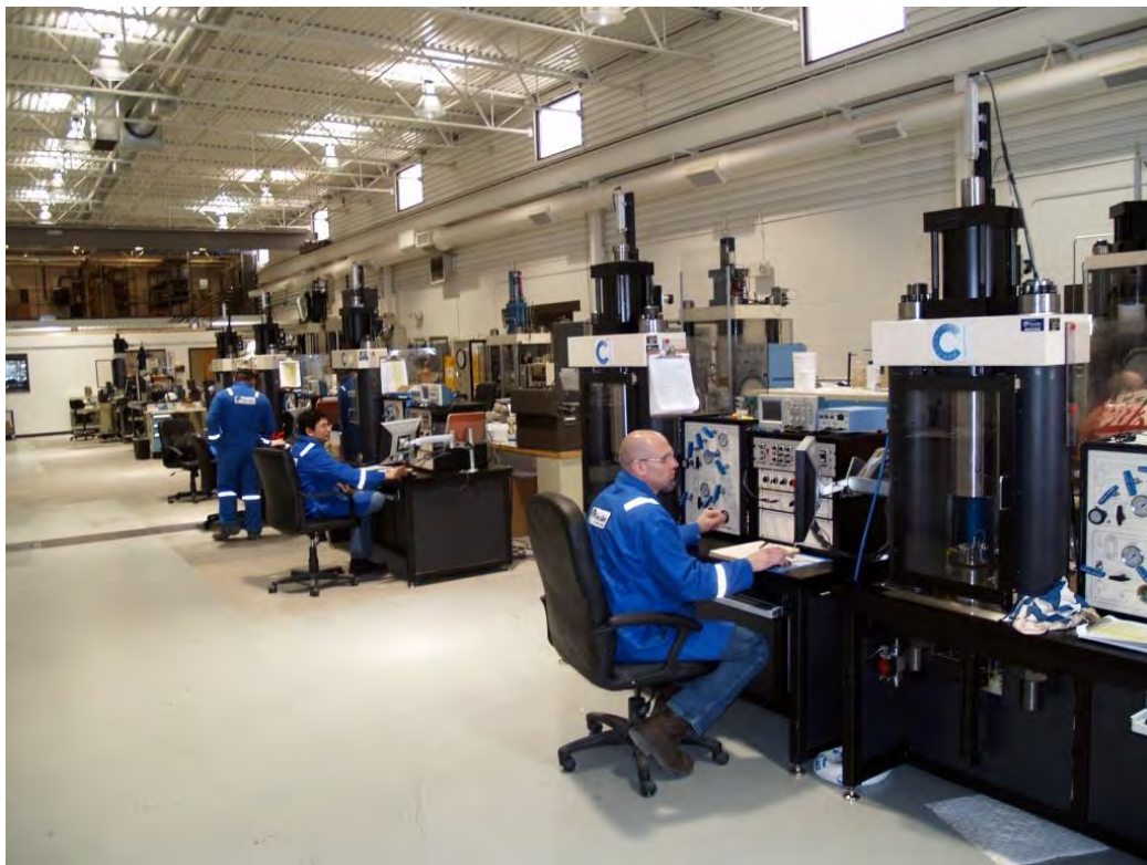
Figure A2 View of part of main Rock Mechanics Lab at TerraTek showing some of the 19 available load frames
