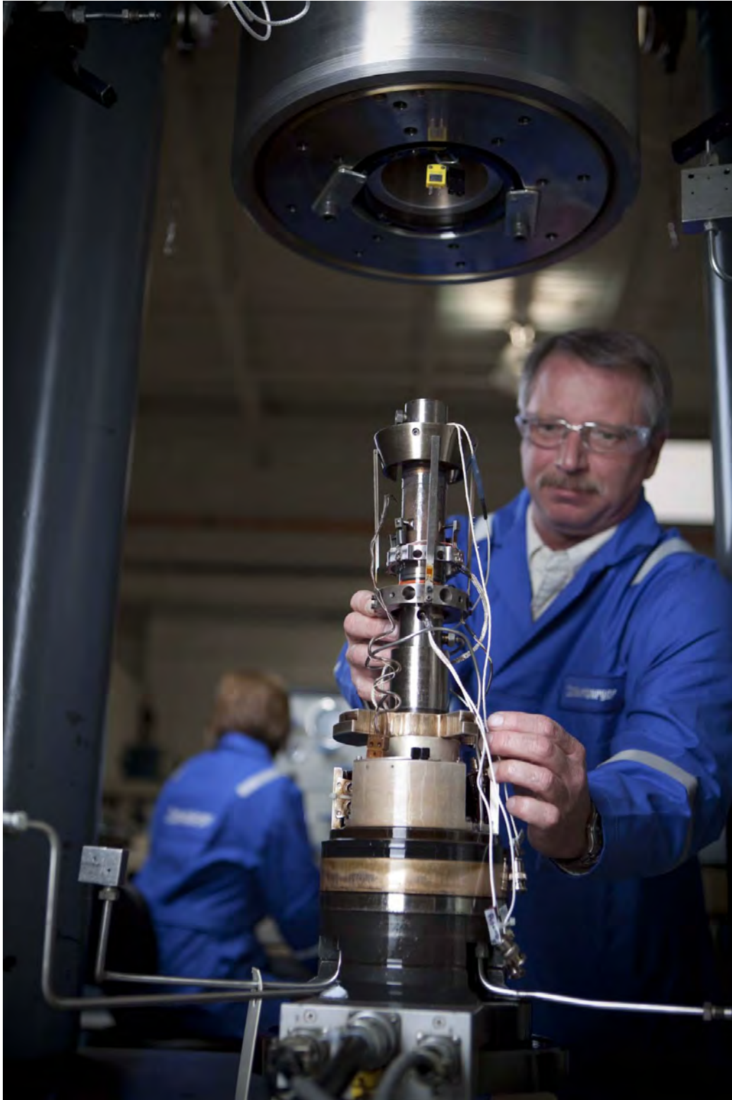
Figure A4 Fully instrumented sample ready to be raised into pressure vessel for triaxial testing.
