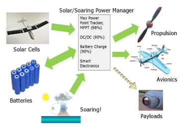
This will optimize product the power conversion from the solar array batteries, batteries from the electronics, and from the batteries to the propulsion motor. The power conversion circuitry will provide state-of-the-art high efficiency power while the microprocessor will run advanced algorithms for maximum power
