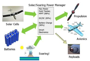
electronics, and from the batteries to the propulsion motor. The power conversion circuitry will provide state-of-the-art high efficiency power while the microprocessor runs advanced algorithms for maximum power point tracking, and an optimized torque motor control to efficiently deliver power to the propulsion system. The conclusion of this
