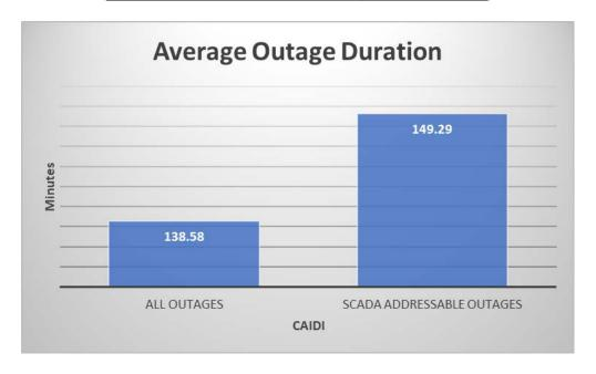
Without having SCADA operation at all of our substations, McKenzie Electric has to dispatch crews to outages that could in the future be restored through SCADA operations. The above numbers reflect our averages from more than 6 years of data. The SCADA addressable outages are events where we could have restored power through SCADA operation.
