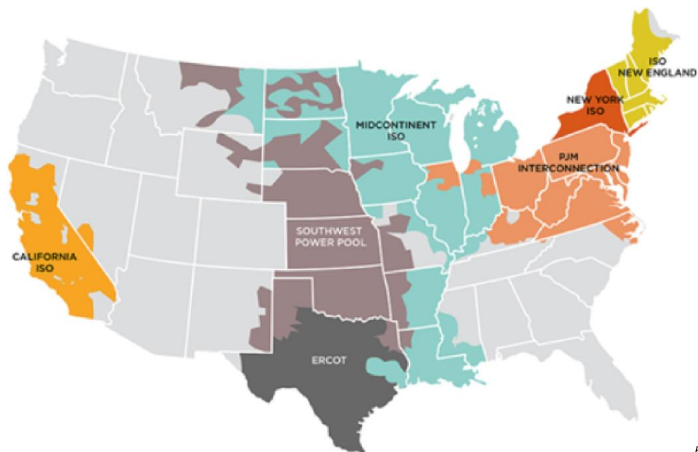
Figure 1. Footprints of U.S. independent system operators (ISOs). MISO also includes Manitoba and Saskatchewan, Canada (Federal Energy Regulatory Commission, 2024).
