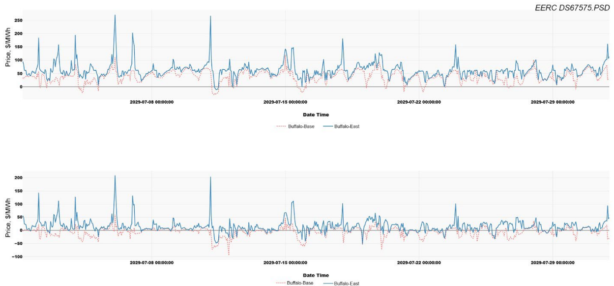
Figure 3. LMP and its congestion component for Buffalo bus under the base case and east scenario – July 2029.
